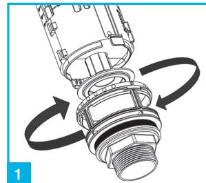
Choose the correct cradle size for the installation, 1 1/2" (factory fitted) or 2". To remove cradle twist and pull from flush valve, to connect reverse procedure.
