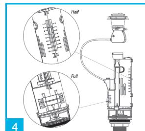
The flush volumes of both the full and half flush can be adjusted to suit your requirements. This is achieved by sliding the adjustment clips.
