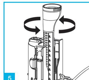
To adjust the overflow tube height, turn tube anti-clockwise and adjust up and down to the correct position. Turn clockwise to lock into place.
