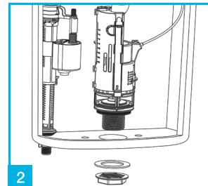
Insert the flush valve into the water tank and tighten to the tank using the washer and nut.
