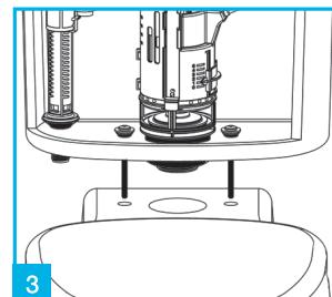
Replace or refit the doughnut washer and fasten the tank to the toilet with the bolt through kit.
