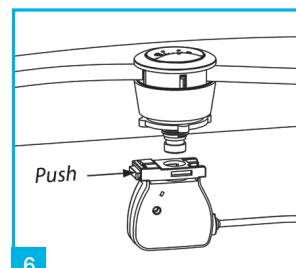
To install the button, insert button into the valves control box while pressing the blue button (see button guide for more information on hole sizes)
