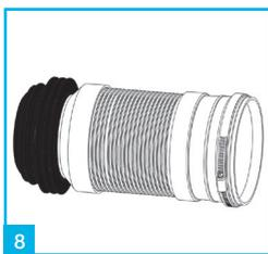
Make waste connections to toilet pan spigot, as per WC pan guidelines. (For back to wall toilet pans, we recommend using a VIVA back to wall flexible pan connector. This connector uses a jubilee locking clip which secures the seal to the pan spigot before positioning the pan into place).
