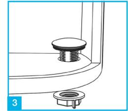
3 For a side entry installation please ensure blanking plug is used in the hole in the bottom
