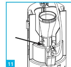
11 To adjust the overflow tube height, turn tube anticlockwise and adjust up or down, we recommend setting the tube to 8.
