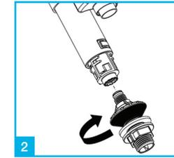
2 To connect, screw the thread into the sprung loaded opening ensuring this is fully secure but not over tightened
