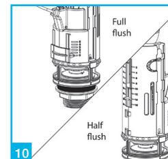
10 The flush volumes of both the full and half flush can be adjusted to suit your requirements. The flush valve is factory set to full flush and a half flush of 3L.
