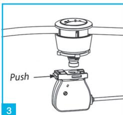
When connecting the button it is very important when deciding on the position that the cable runs smoothly, this prevents valve failure. Once the position of the button is decided fix into position as shown. Please note the hole size for the button in 40mm.
