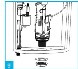
9 Insert the flush valve into the cistern and tighten using the washer and nut.
