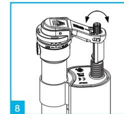
8 Set the lifted float to the same height as the 6L mark on the cistern by turning the adjustment screw (clockwise for more water and anticlockwise for less water).
