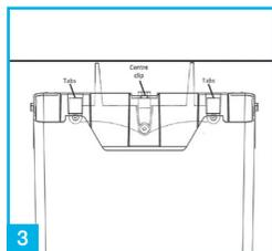
To hang the cistern, ensure the bracket is firmly fixed, slowly lower the cistern holding it centrally to the bracket. Ensure the tabs are aligned with the recesses in the cisterns, push down firmly until cistern clicks into place.
