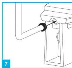
With the toilet pan in position push to flush cone into the WC toilet inlet
