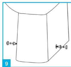
Double check all connections, i.e. water feed to inlet connection, flush valve to flush pipe connection, flush pipe to pan connection and pan spigot to waste connection. Once happy they are all water tight, tighten and secure WC pan.
