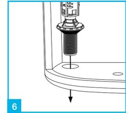
6 Remove the plastic washer and nut from the thread and place the valve into the desired hole in the cistern ensuring the conical rubber seal sits evenly inside the hole
