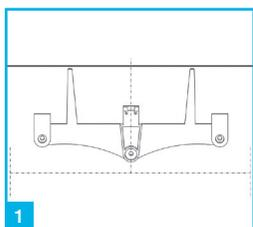
Position and fix the support bracket in the centre of the unit or in line with the WC waste outlet. The guide tabs should be level and underneath the top of the unit. This allows ample clearance for lid to be removed and parts to be accessed.
