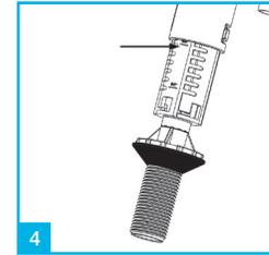
4 To adjust the height twist the valves base 1/8 turn clockwise and adjust the height to the correct level. We recommend setting the valve at 9.5.
