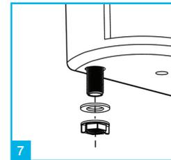
7 Secure the valve to the cistern by replacing the plastic washer and screwing the nut to the thread. Do not over tighten.
