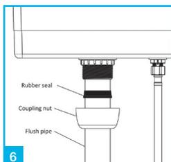
Once cut to size, connect the flush pipe to cistern using rubber seal and connection nut and fit the flush cone onto narrow end of flush pipe.
