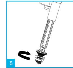
5 Once the correct height is achieved, twist the base back 1/8 turn anticlockwise. At this point the valve is ready for installation
