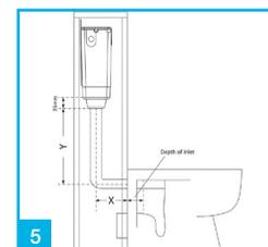
Position the WC pan, and check measurements for the flush pipe. Cut the flush pipe to size if required. It is important to remember that 35mm needs to be inserted into flush valve thread and again a certain amount depending on WC pan needs to project into toilet inlet.
